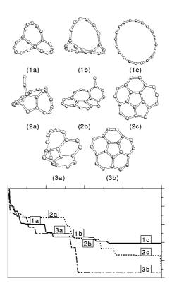
FIG. 2. Running the genetic algorithm on  $C_{20}$ . The solid line shows the generic lowest energy structure when the algorithm is run with no mutation ( $\mu = 0$ ); the structures (1a) - (1c) are present in the population at the times indicated. Essentially all ecologies get trapped in monocyclic rings (1c). The dashed line (structures (2a) - (2c)) and the dot-dashed line (structures (3a) and (3b)) illustrate the results when mutation is added ( $\mu = 0.05$ ).
